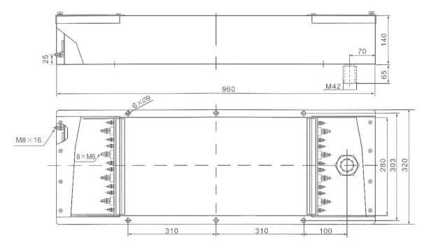
(Note: The power connection studs are M6 for the 16 - 70 A version and M8 for 100A version)
