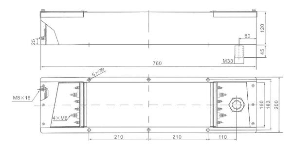
(Note: The power connection studs are M6 for the 16 - 70 A version and M8 for 100A version)
