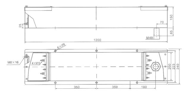
(Note: The power connection studs are M10 for the 150A and 200A versions)
