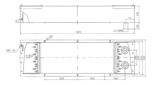
(Note: The power connection studs are M10 for the 150A and 200A versions)
