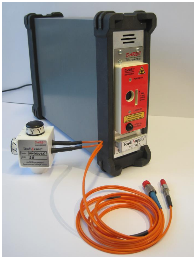
Figure 2: Beam shutter (red) on the RadiSupply® plug-in card (in the RadiCentre® system)
