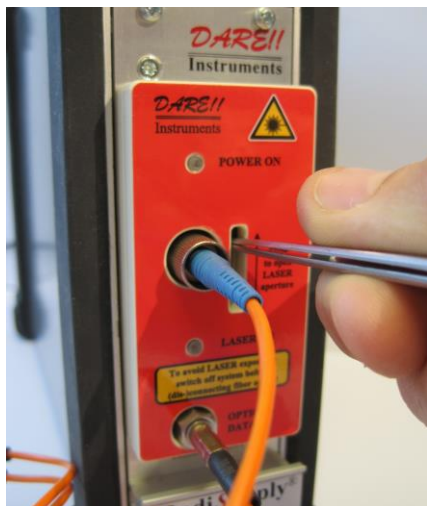
Figure 5: Both the FC connector (top) and FSMA connector (bottom) are connected to the beam shutter
